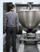
DED-produced Ø1.2m Combustion Chamber
